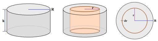
The left image shows the cylinder and its dimensions (R and h).
