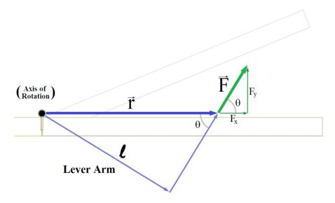
If we apply a force  $\vec{F}$  to an object, we define the vector  $\vec{r}$  to start at the axis of rotation and at the position where the force is applied.  $\theta$  is defined to be the angle between  $\vec{F}$  and  $\vec{r}$ .
