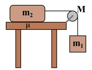
**Example**: A box of mass  $m_2 = 10.0$  kg sits on a table as shown. On one side a cord connects it to a hanging weight of mass  $m_1 = 25.0$  kg. The cord stretches over a frictionless pulley, a solid disk of uniform density with mass M = 5.00 kg. If the coefficient of kinetic friction between the box and table is 0.300, determine the acceleration of the box on the table.
