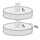
**Example**: A solid disk ( $I_1 = 4.00 \text{ kg} \cdot \text{m}^2$ ) is spinning about a fixed spindle at  $\omega_0 = 15.0 \text{ rad/s}$ . A second solid disk ( $I_2 = 6.00 \text{ kg} \cdot \text{m}^2$ ), which is not rotating, is placed on the spindle and dropped onto the first disk. There is friction between the two disks, and eventually they spin together. Determine (A) the velocity of the two discs once they start spinning together and (B) the energy is lost during the collision.
